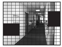
This sub-menu shows the camera's view broken up into a grid. You choose which sections of the image detect motion.
